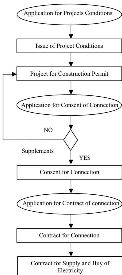
**Figure 2:** Procedure required for Connection to the grid.
