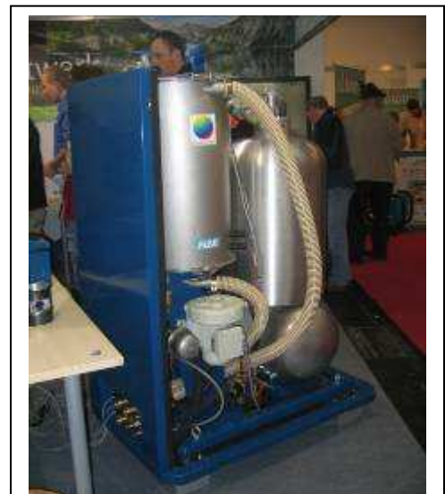
A wood pellet sterling machine that definitely has a future in Sweden
